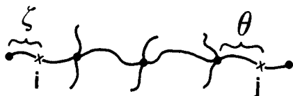
Figure 3. Two points i and j of the network separated by d = 3\phi -functional junctions (where \phi = 4 ). The position of points i and j are measured with respect to the nearest \phi -functional junction from the left in units of the length of the chain contour between \phi -functional junctions.
